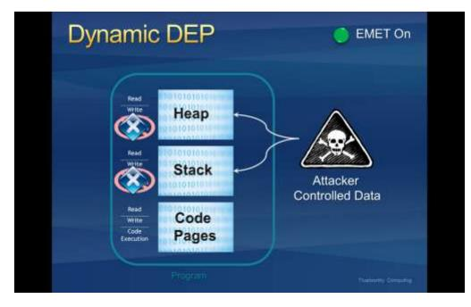
Figure 4: DEP blocking shellcode from running
