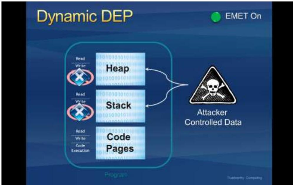
Figure 4: DEP blocking shellcode from running
